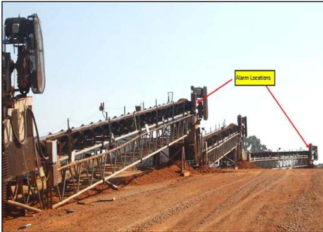
**Figure 8:** “Piggy-Back” conveyors are 100 foot conveyor segments designed to be easily reconfigured to move materials from the active pit to the field conveyor.
