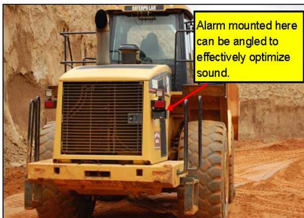
**Figure 7:** Photograph showing installation location of bbs-107 on a 980G loader.
