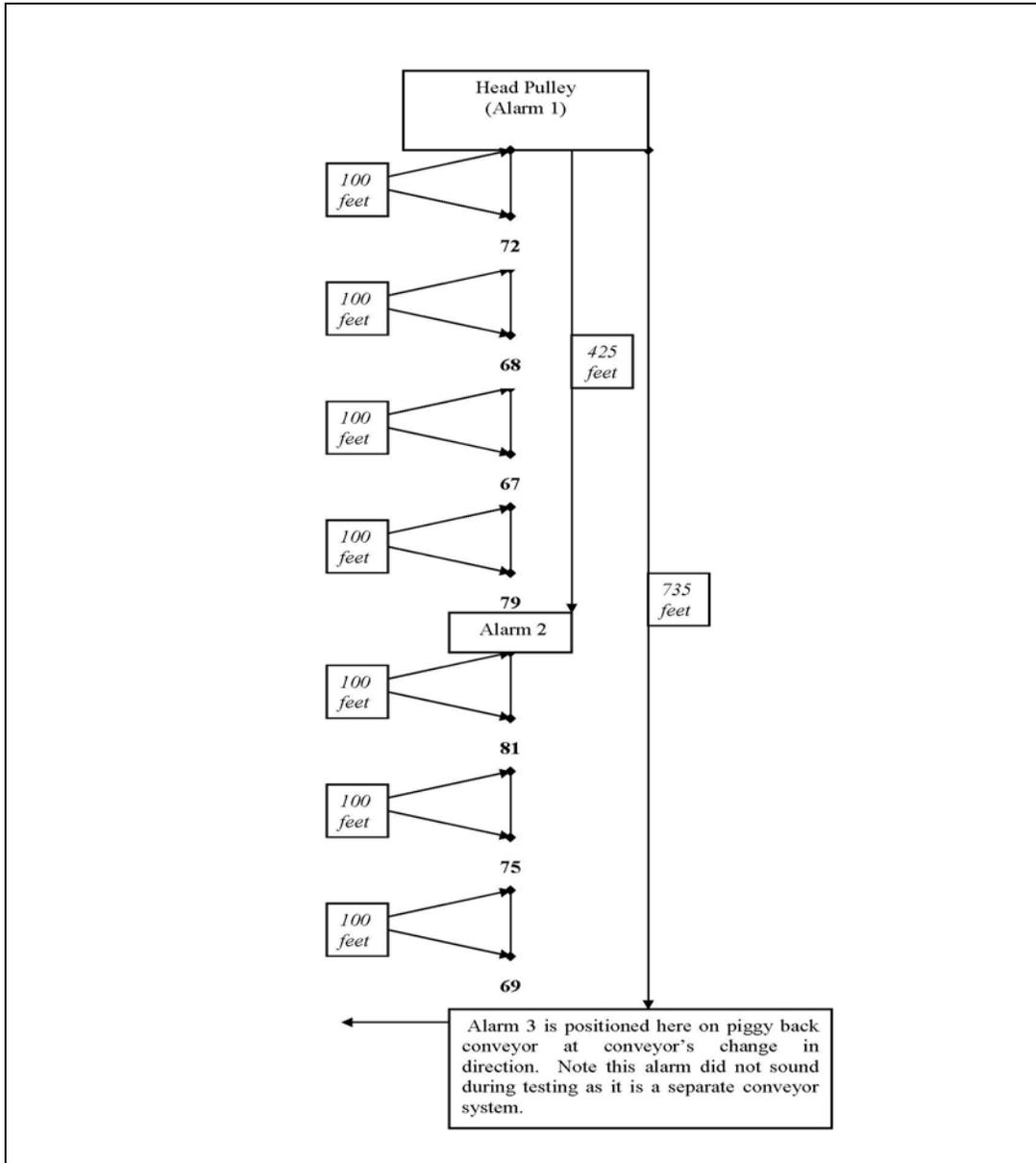
**Figure 9:** Field conveyor with two alarms. Note that the alarms sound simultaneously when started. Sound measured at 100 feet intervals. Distance stepped off by foot and estimated. All measurements in dB(A).
