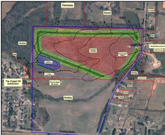
**Figure 2:** Berm constructed around mining operations. Note the close proximity (~500 feet) from the nearby subdivision to the bottom-left of the photo.
