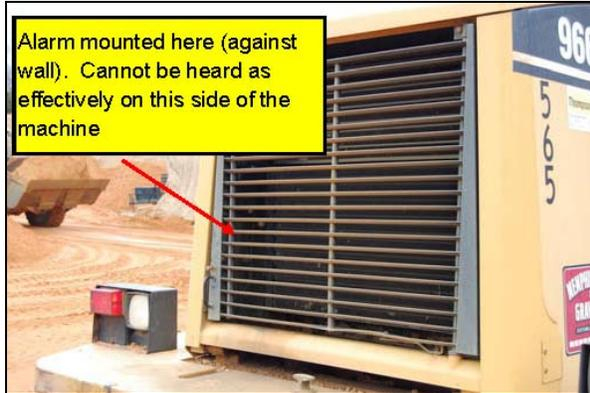
**Figure 6:** Photograph showing installation location of bbs-107 on a 966G loader. This location is not optimal and should be rearranged.
