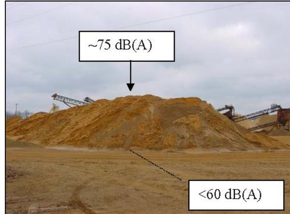
**Figure 3:** A stockpile of fill sand is placed between plant operations and the property boundary. The sound measures below background levels when measured on the side away from the plant.
